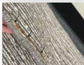
Back edge view, glue along the edge to try to hold the rug together.
