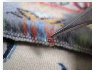
A "hand knotted" rug is cut open to show the interior fibers and the wool knot that is tied around two warps. These knots cannot be pulled away from the rug without cutting it open first.
